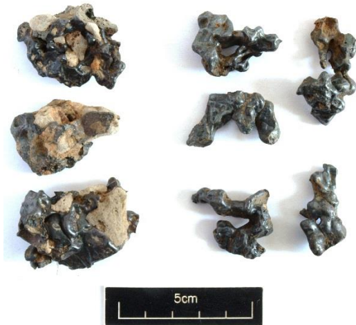
Figure 4. Flow slag (right) and flow slag with vitrified ceramic lining (left) from NEW-EX-18 (6138)
